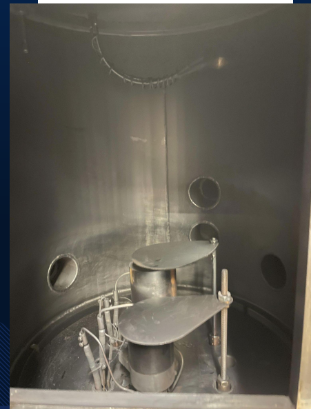
CdS/CdSe Evaporation Chamber
